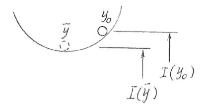
An equilibrium state  $\bar{y}$  with potential energy  $I(\bar{y})$ . A perturbed state  $y_0$  with potential energy  $I(y_0)$ .
