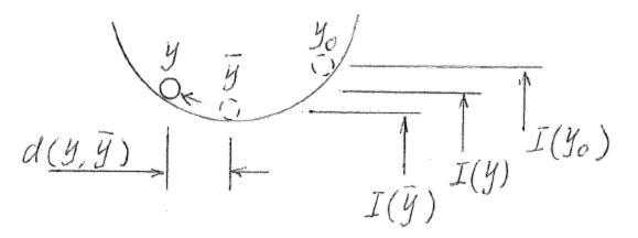
An equilibrium state  $\bar{y}$  with potential energy  $I(\bar{y})$  A perturbed state  $y_0$  with potential energy  $I(y_0)$ . The ensuing motion y with potential energy  $I(y_0)$
